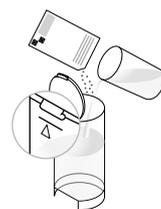
**3** **Pour 1 Nespresso descaling** liquid sachet into the water tank. Fill the water tank up to the 0.6 L line with fresh drinking water.
