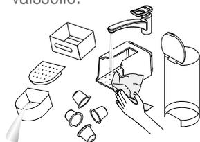
**1 Empty the drip tray, the drip base and the capsule container every day.** Also remove the water tank with its lid and clean them all with odorless detergent and rinse with warm / hot water.
